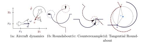
Fig. 1: Roundabout maneuvers for collision avoidance in air traffic control
