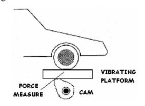
The validation criteria is simply the ratio between the minimal measured force between the wheels and the platform, and the static force, which is simply the weight of the car. As this ratio tends towards 0, the vehicle tends to lift off the platform and the tires stop transmitting the force of the motor to the road because of the lack of friction (e.g. the force between wheels and platform becomes too small).
