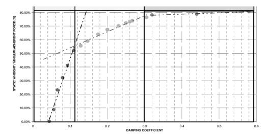
The conclusions of the study are that the component that has the most influence on dynamic behaviour of the suspension system is the shock absorber (e.g. the damping ratio), and that a 'Limit Damping Coefficient' as validation criteria can be established, below which the dynamic behaviour of the suspension system demonstrates an outstanding loss of performance. That means an excessive wearing out of the shock absorber and a need to change it in order to maintain proper vehicle safety conditions.
