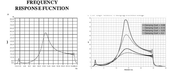
The result show that the minimum adherent force becomes dangerously close to 0 as the damping ratio drops below 0.1.
