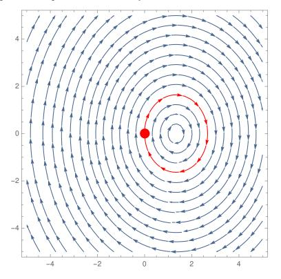
From the plot, it is easy to see that the maximum horizontal position of the box is  $x \leq 2\frac{c}{k}$ . If we tried to prove this right away with dI, we would fail. The technique we have been using so far of cutting in extra invariants would not work either: it tells us to cut in  $v \leq 0$ , which would not be provable for the above system.
