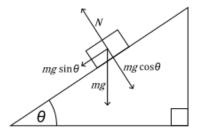
From the picture, we see that the box is being driven parallel down the slope by a force  $mg\sin(\theta)$ . For our purposes, we shall work with accelerations and so we will assume that the box has unit mass, i.e., with m = 1.
