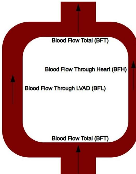
Figure 2: Modelling flow as pipes
