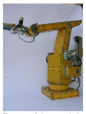
The structure of robot arms can be discussed in a general fashion. Robot arms are made up of links and joints. The joints may either be prismatic, meaning that they extend forward in the direction of the joint it is attached to, or rotational, meaning that they change the angle between the links they are connected to. By combining these in different arrangements, it is possible to create any number of robot arms. For example, the Stanford arm contained 3 rotational joints.
